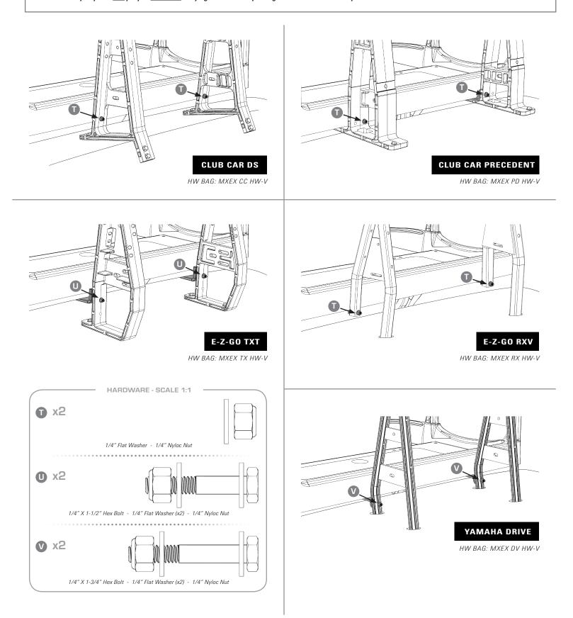
NOTE: Fully tighten Rear Seat Kit Brackets and Bumper Angle Hardware.
